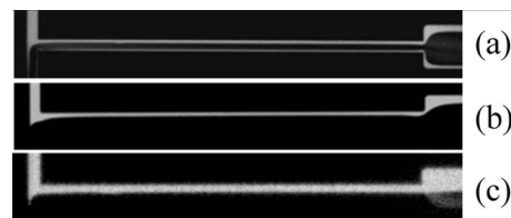
FIG. 9. Threading in head-on microfluidic channels. (a) Q_w = 0.5Q_o = 0.5 \mu\text{l}/\text{min} , (b) Q_w = Q_o = 0.75 \mu\text{l}/\text{min} , and (c) Q_w = 2Q_o = 1 \mu\text{l}/\text{min} .
