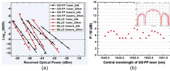
Fig. 5. (a) BER curves; (b) P/W ratio as the central wavelength of GS-FP laser varies within the 3-dB reflecting spectrum of SSFBG (shown in the inset).
