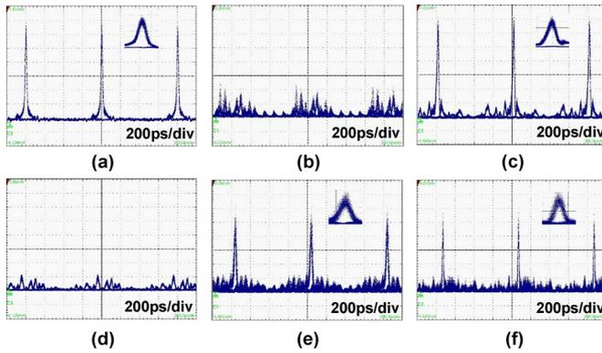
Fig. 4. Eye diagrams. The case of GS-FP laser: (a) modulated signal before the encoders; (b) encoded signals for the case of two users; (c) signal after matched decoding; (d) signal after mismatched decoding; (e) decoded signal after 20-km transmission, two users. For comparison, the case of MLL (f) decoded signal after 20-km transmission, two users.
