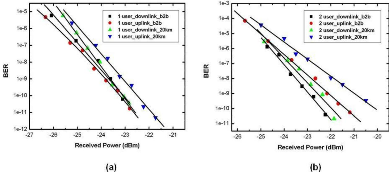
Fig. 5. BER curves in the case of (a) one user; (b) two users.
