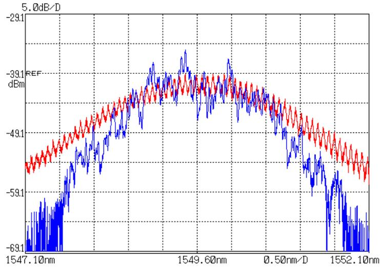
Fig. 3. Spectra of OCDMA coded signals (the lower one) and clock pulses (the upper one).
