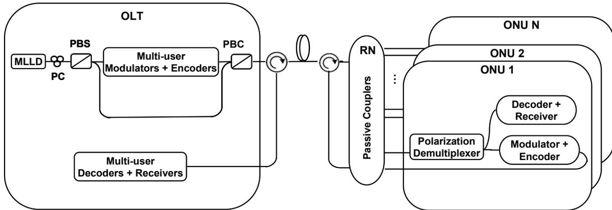
Fig. 1. Centralized light source OCDMA PON based on polarization multiplexing. MLLD: mode locked laser diode; PBC: polarization beam combiner; PC: polarization controller.
