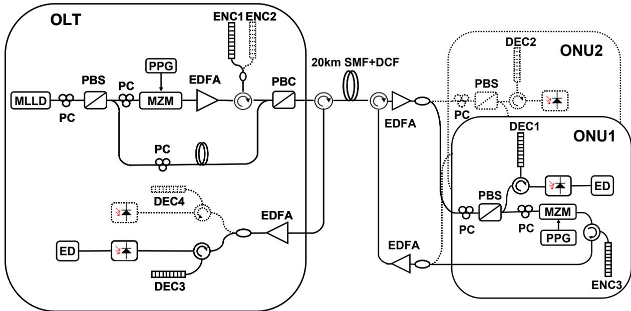
Fig. 2. Experiment setup. MZM: Mach-Zehnder modulator; PPG: programmable pattern generator; SMF: single mode fibre; DCM: dispersion compensation module; EDFA: erbium doped fibre amplifier; PBS: polarization beam splitter; ENC: encoder; DEC: decoder; ED: error detector.
