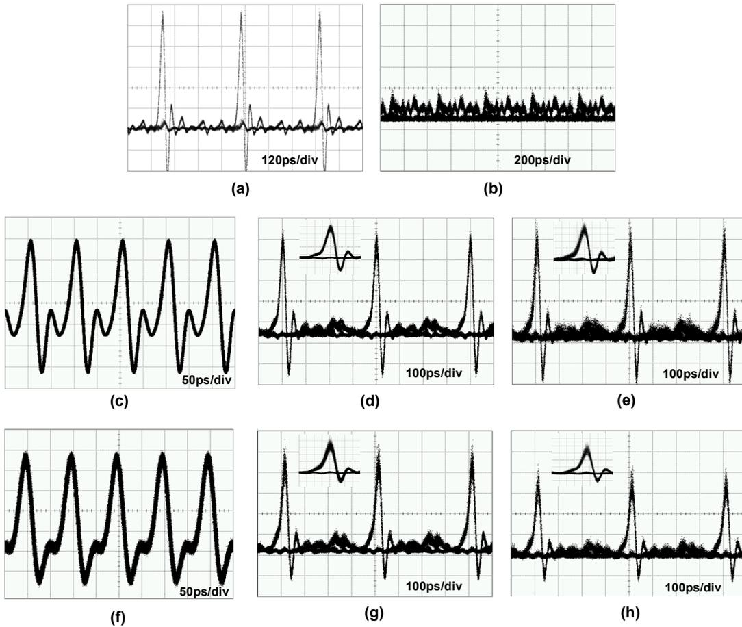
Fig. 4. Eye diagrams for (a) modulated signal before encoders; (b) encoded signal in the case of two users; (d) decoded downlink signal in the case of one user; (e) decoded downlink signal in the case of two users; (g) decoded uplink signal in the case of one user; (h) decoded uplink signal in the case of two users. Clock pulses (c) generated from MLLD; (f) received at the ONU.
