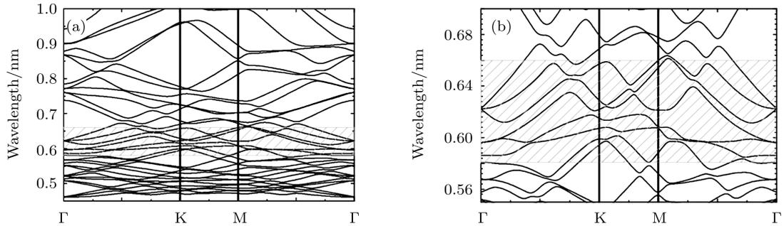
**Fig.2.** (a) Band structure of 2D triangular lattice of air holes in the HCPCF. (b) Enlarged band diagram in visible region. In both cases, the shadow area indicates the wavelength range corresponding to the emission band of the luminescent microparticles.
