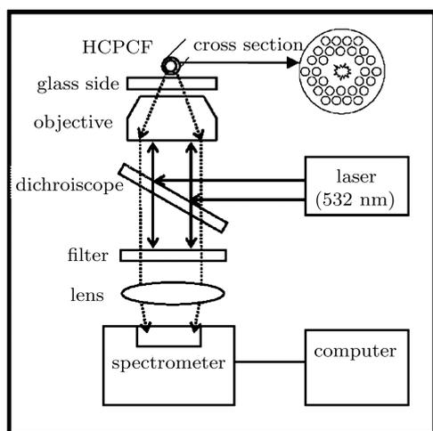
**Fig.4.** Schematic showing the experimental setup used to investigate the spontaneous emission modification of luminescent microparticles induced by an HCPCF.
