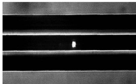
**Fig.5.** Photograph of the HCPCF with inserted luminescent microparticles.
