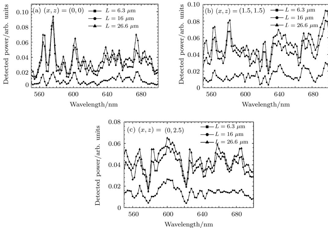
**Fig.3.** Wavelength dependence of the detected power for a point source located at different positions in the central hole of the HCPCF. (a)  $(x, z) = (0, 0)$ ; (b)  $(x, z) = (1.5, 1.5)$ ; (c)  $(x, z) = (0, 2.5)$ . The size of the power detector  $L$  corresponds to the numerical aperture of the objective lens used in the experiments.
