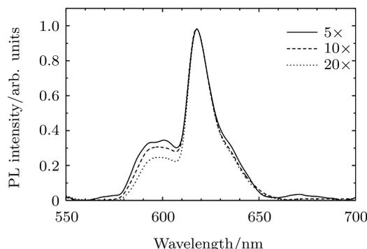
**Fig.6.** PL spectra for microparticles on a glass slide measured by objective lenses with different magnifications.
