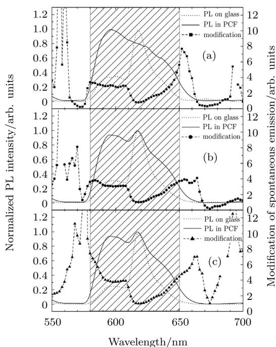
**Fig.7.** PL spectra for microparticles located in the HCPCF measured by objective lenses with different magnifications. (a) 5 $\times$ ; (b) 10 $\times$ ; (c) 20 $\times$ . In each case, the PL spectrum for microparticles placed on a glass slide is also provided for reference. Both of them are normalized in order to compare the spectral shape.
