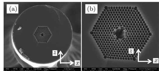
**Fig.1.** SEM images for the cross sections of the HCPCF (a) and the enlarged 2D PC structure (b).
