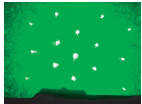
Fig. 2. Diffraction pattern of the optical matter obtained at the optimum trapping power of about 100 \text{ mW} . It was projected on a screen placed several centimeters away from the sample cell.
