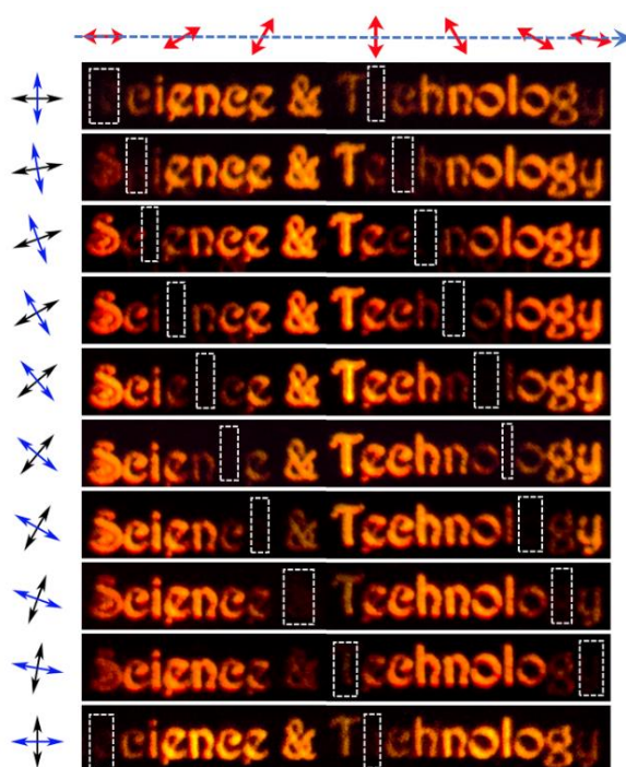
Figure S11. Recording of the polarization states of femtosecond laser light into different characters of Science & Technology with an increment of 10^\circ and a pixel size of 0.50\ \mu\text{m} .
