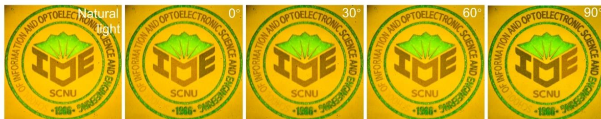
Figure S17. Colorful school logo created by using continuous wave laser light at 750 nm and observed by using unpolarized (1 st column) and polarized white light with polarization angles of 0° (2 nd column), 30° (3 rd column), 60° (4 th column), and 90° (5 th column).
