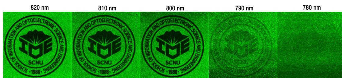
Figure S7. Pattern recorded by using 800-nm femtosecond laser pulses ( 0.67 \text{ mJ/cm}^2 ) and extracted by using femtosecond laser pulses with different wavelengths ( 0.17 \text{ mJ/cm}^2 ).
